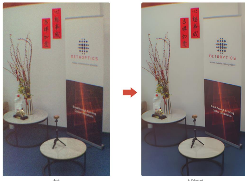
Figure 5: Image quality after channel overlay and other basic processing versus additional AI processing. Left: base processing showing a high-quality rectangular metalens color image. Right: after AI processing, with substantially improved clarity and detail. (Source: MetaOptics Technologies)
