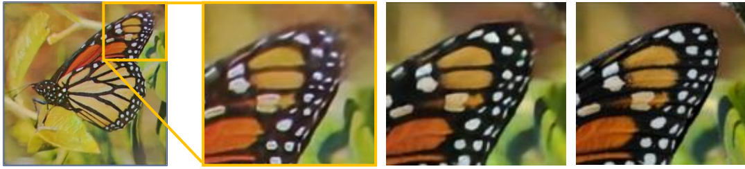
Figure 4: Left: Image with zoom-in showing peripheral image distortion without the Spatial-Aware Attention Scheduler; center: Image restoration with the Spatial-Aware Attention Scheduler; right: Ground Truth image.
