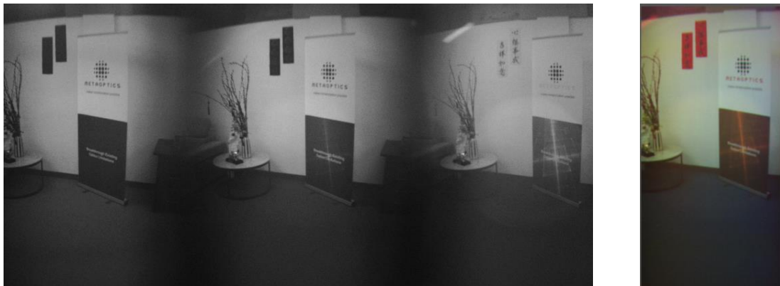
Figure 2: Rectangular metalens image fusion. Left: Raw monochrome sensor frame from MetaOptics RGB metalens camera containing blue, green, and red monochromatic images of the same scene before fusion to a raw color image. Right: after the fusion stage where the three sub-apertures are aligned and combined into the raw color image.
